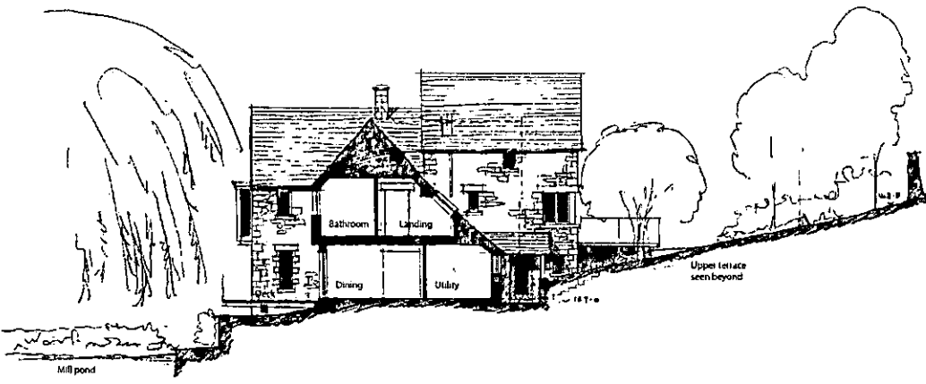
Section DD - Looking west towards entrance wing
